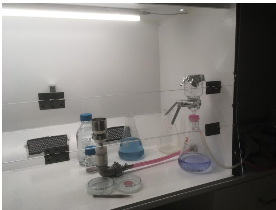
Figure 8: Filtering equipment inside the blower box, RSI lab (RSI, 2019)
